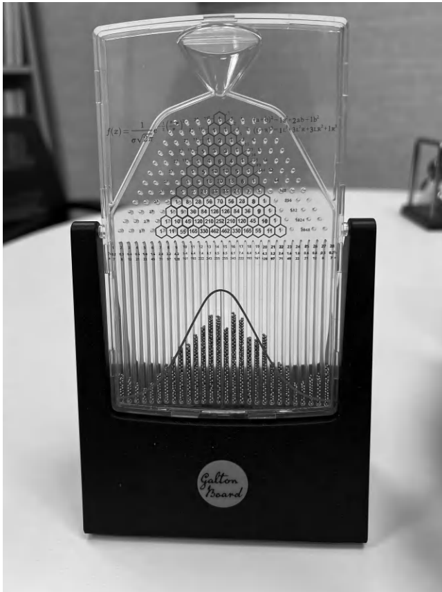
Figure 5.1 A Galton board, similar to the large ones that are installed in museums for visitors to interact with and observe.
